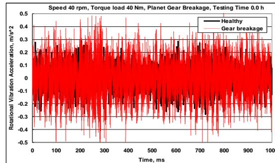
Fig. 8 Time-domain rotational vibration acceleration (40 rpm 40Nm)
