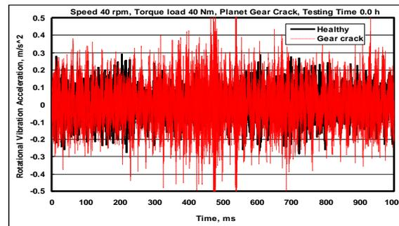
Fig. 4 Time-domain rotational vibration acceleration (40 rpm 40Nm)
