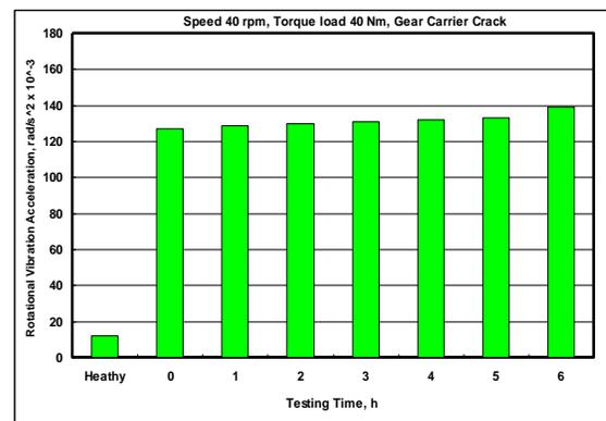
Fig. 11 RMS value rotational vibration acceleration (40 rpm 40Nm)
