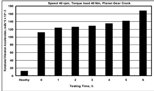
Fig. 5 RMS value rotational vibration acceleration (40 rpm 40Nm)
