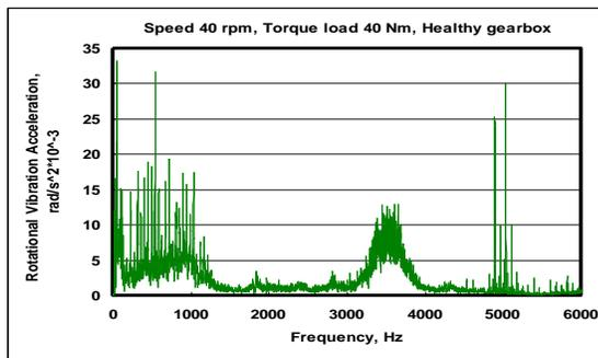
Fig. 3 Frequency-domain rotational vibration acceleration (40 rpm 40Nm).
