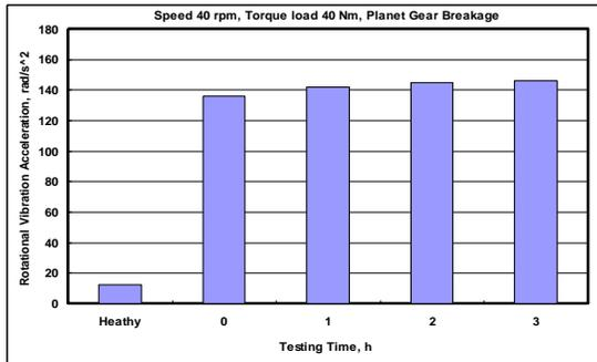
Fig. 9 RMS value rotational vibration acceleration (40 rpm 40Nm)
