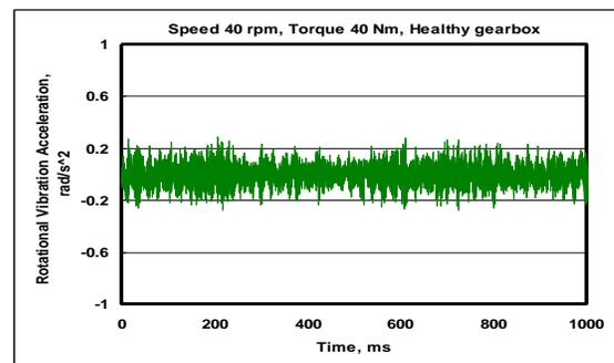
**Fig. 2** Time-domain rotational vibration acceleration (40 rpm 40Nm).
