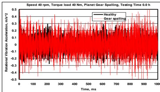
Fig. 6 Time-domain rotational vibration acceleration (40 rpm 40Nm)
