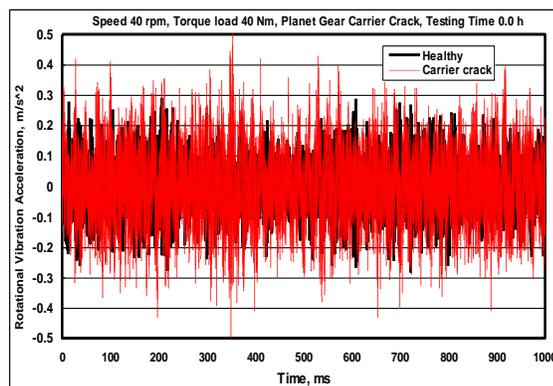
Fig. 10 Time-domain rotational vibration acceleration (40 rpm 40Nm)
