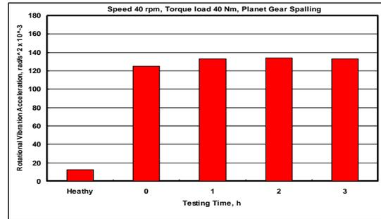
Fig. 7 RMS value rotational vibration acceleration (40 rpm 40Nm)
