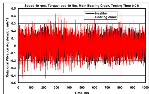
Fig. 12 Time-domain rotational vibration acceleration (40 rpm 40Nm)
