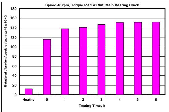
Fig. 13 RMS value rotational vibration acceleration (40 rpm 40Nm)
