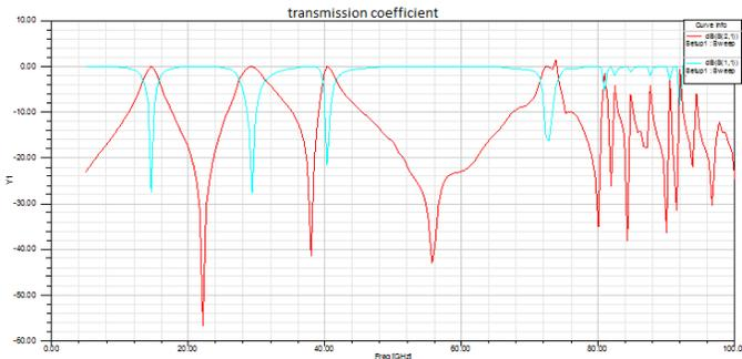
Fig 6 Frequency response curve for scaling factors of 2 and 5
