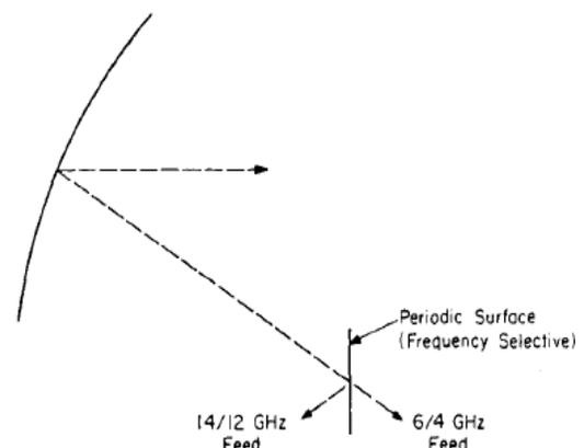
Fig 2. Reflector antenna system using frequency selective screen.
