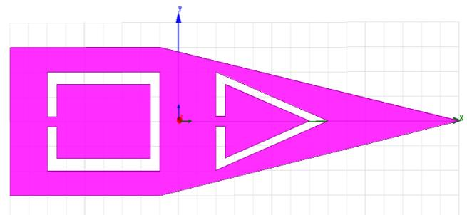
Fig 1: Proposed Patch Structure
