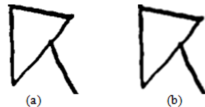
Fig 4. Results of smoothing algorithm to the character « R »; (a) input letter; (b): after smoothing
