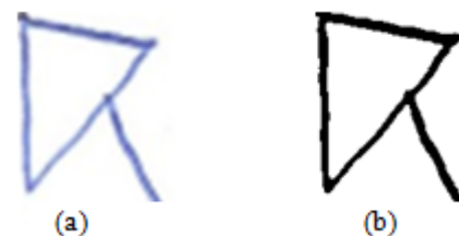
Fig 3. Results of binarization Otsu algorithm to the character « R » (a) input letter; (b): binarization (level=0.8196)
