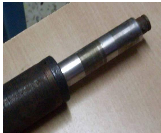
Figure 1.1 Worn out bearing surface of the Rotor, (Courtesy VIRA PUMPS)
