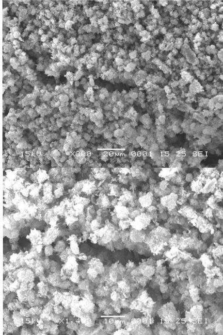
Fig.1 SEM images of NZVa: a) at 20 µm / 200 X. b) at 10 µm / 1000 X
