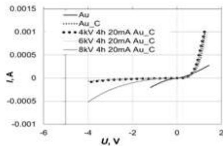
**Fig. 4.** Volt-Ampere characteristics of pnjunctions
