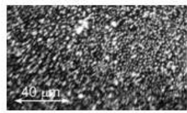
**Fig. 2.** Silicon carbide precipitates
