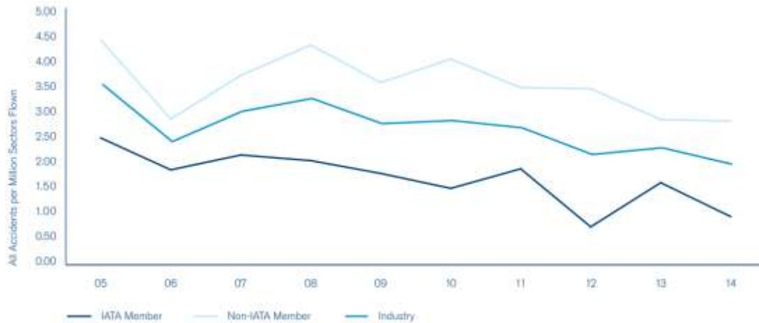
Fig. 7. All Aircraft Accident Rate (IATA Member Airlines vs. Industry, 2005-2014): includes substantial damage and hull loss accidents for jets and turboprops (IATA, 2015)
