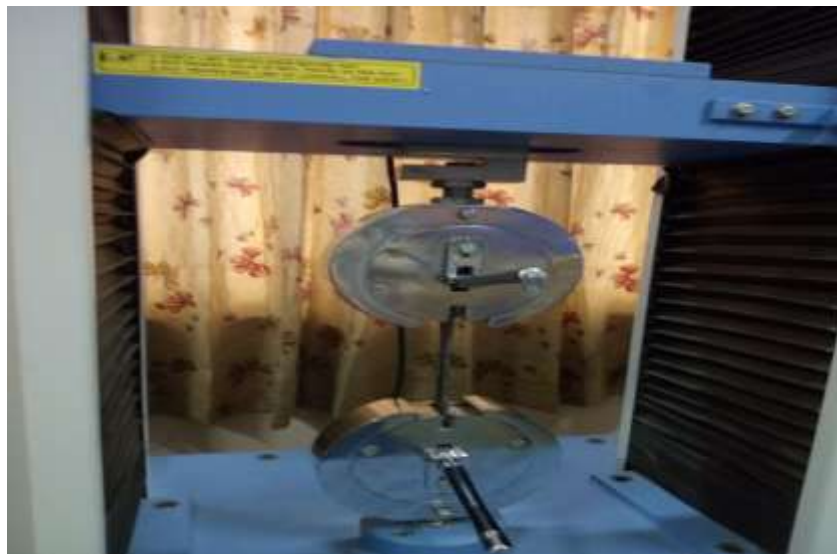
Figure 1. UTM with Tensile test specimen
