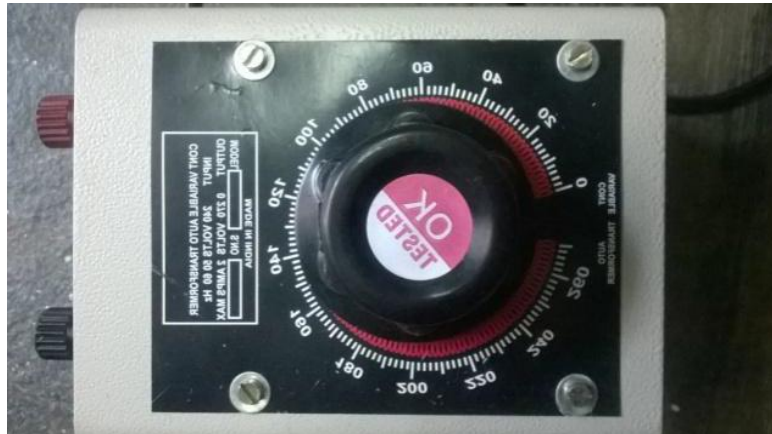
Figure 4: Dimmer start for variable speed to stirrer
