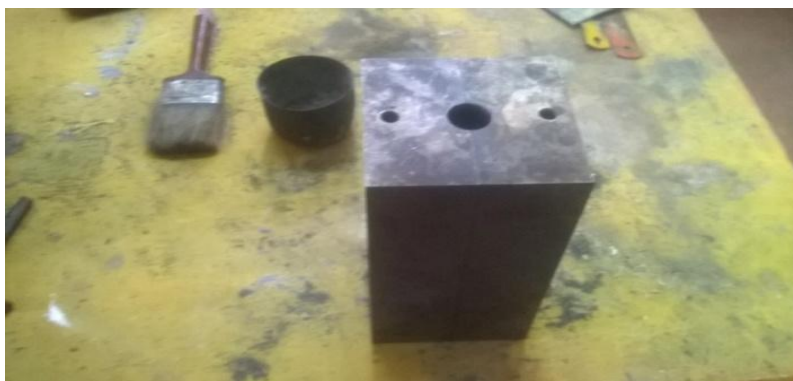
Figure 5: Mould preparation for Metal matrix composites
