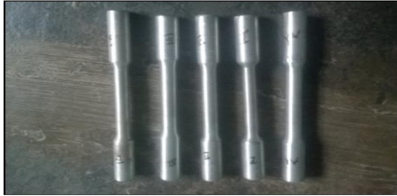
Figure 6: Fabricated hybrid metal matrix composites
