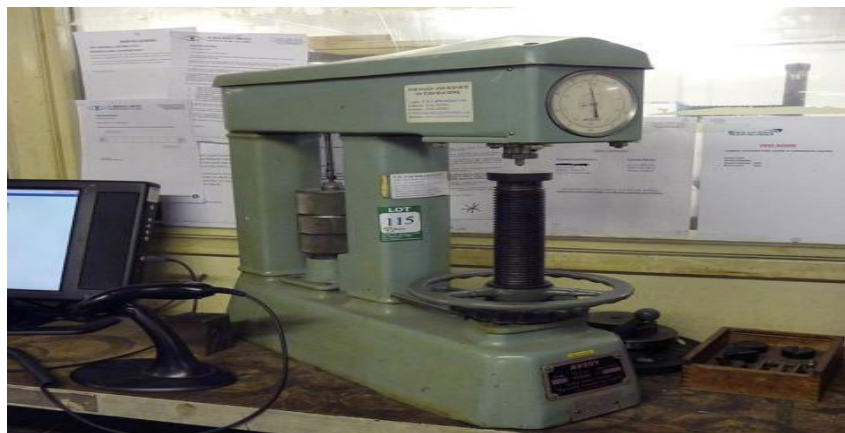
Figure 8: Computerized Brinell hardness equipment
