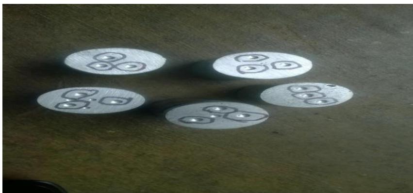
Figure 9: Dents formed during hardness method
