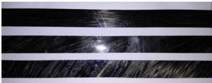
Figure 7: Carbon epoxy composite beams in fiber orientation 0^{\circ} , 30^{\circ} and 60^{\circ}
