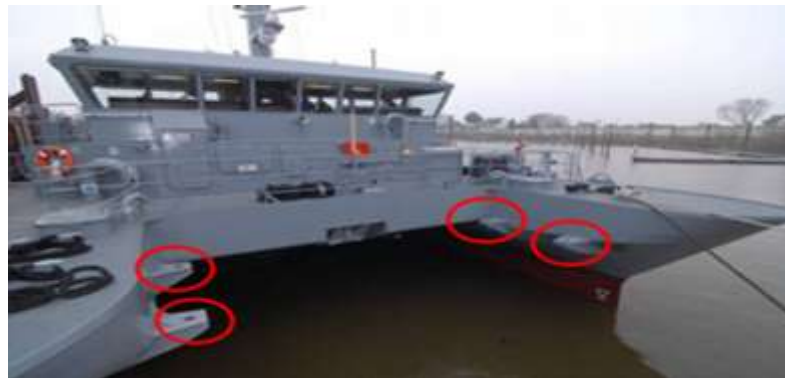
Fig. 2. In-built brackets for installing single 20 ft. standard container.
