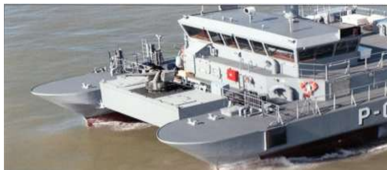
Fig. 3. Artist's impression of a small-caliber naval gun installed on platform of TEU 20' standard container.
