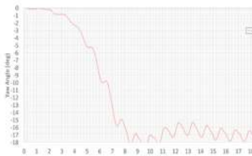
Fig. 22: Exponential Increase of the Yaw Angle of the OPV; Wavelength = 6.8m
