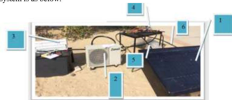
Figure 2.9. Solar Air Conditioning system.
