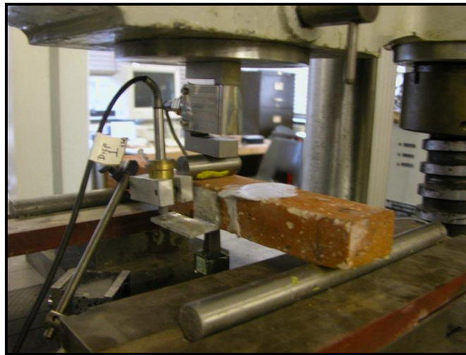
Plate 3 - Set up for half scale model unit fracture test.
