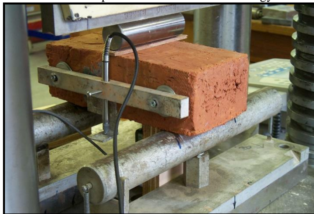
Plate 2 - Set up for single brick unit fracture energy test.
