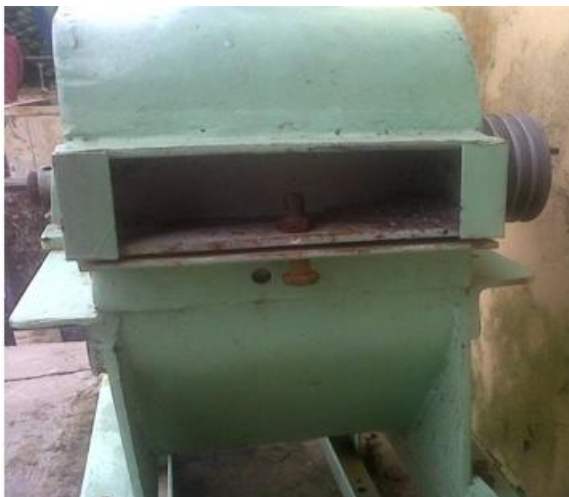
Plate 3: safety hollow opened
