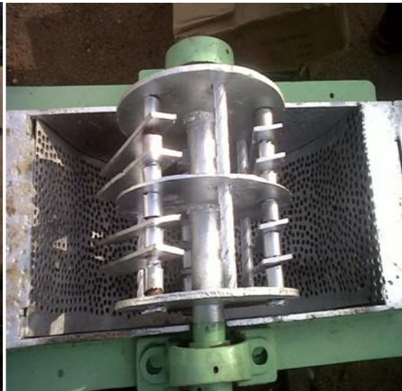
Plate 2: hammers on the auxiliary shafts
