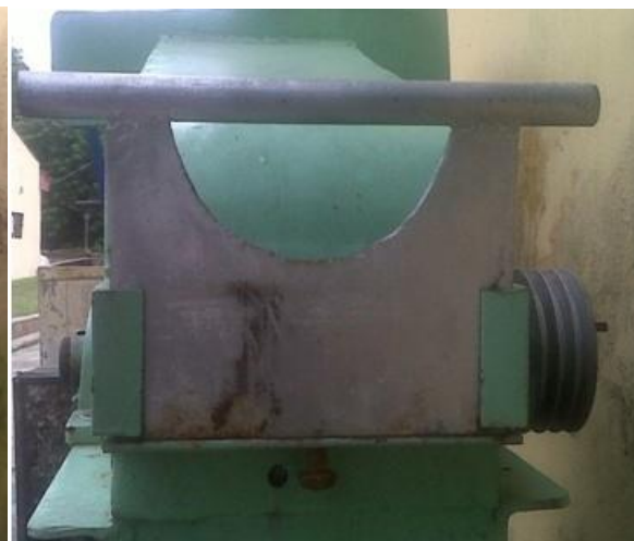
Plate 4: safety hollow closed with mild steel
