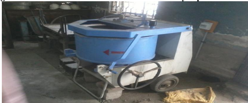
Figure 3: Concrete Mixer used in Laboratory
