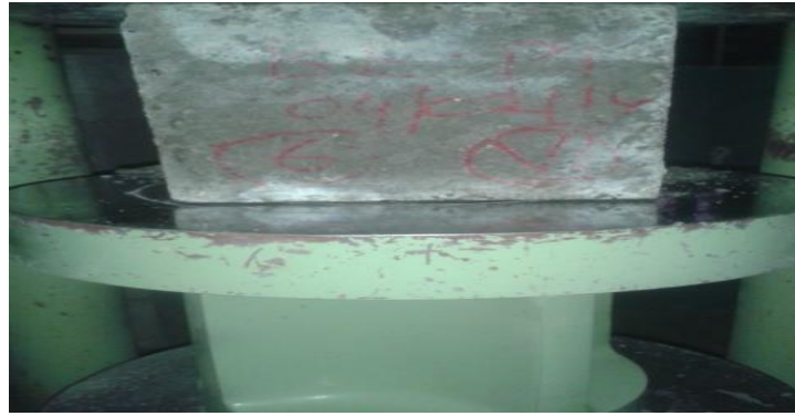
Figure 5: Compression Test on Concrete Cube (UTM Machine)
