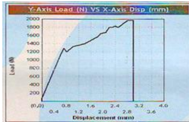
Fig5: variation of load with respect to deformation in 3 layered Glass-Jute-Glass specimen
