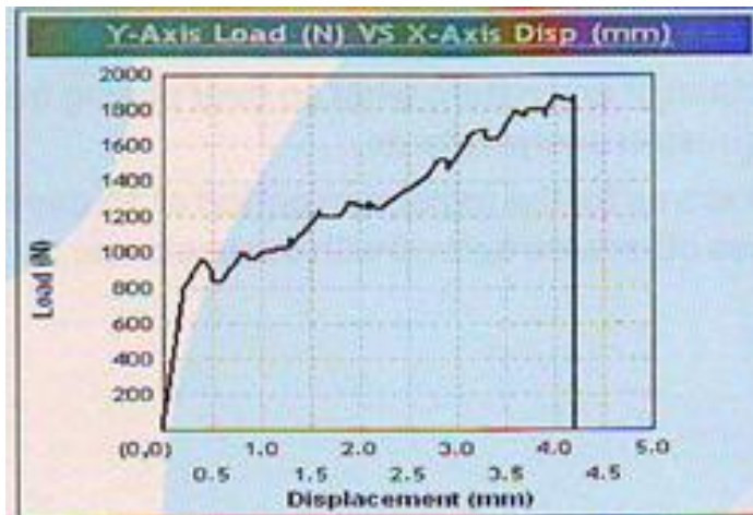
Fig6: Variation of load with respect to deformation in 3 layered Jute-Glass-Jute specimen.
