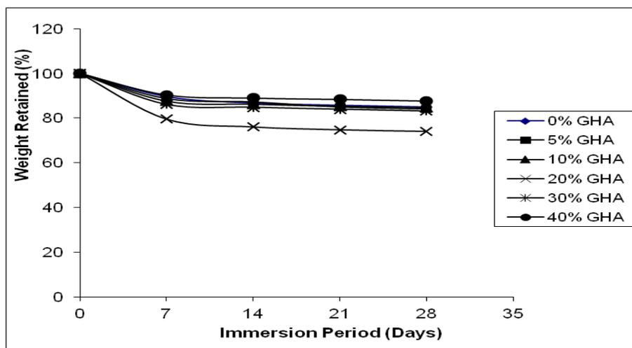
Figure 8: Weight of GHA-Concrete immersed in  $HNO_3$  medium
