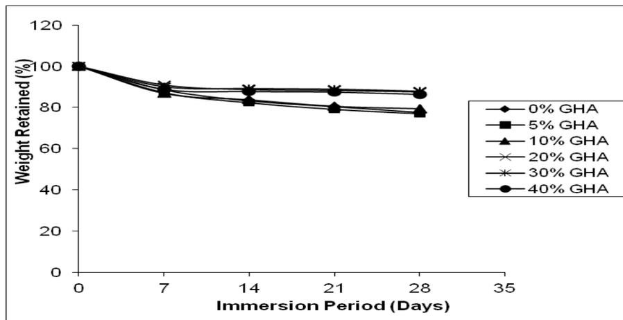
Figure 7: Weight of GHA-Concrete immersed in  $H_2SO_4$  medium.
