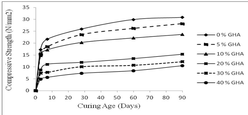
Figure 2: Compressive strength of GHA- Concrete grade 20
