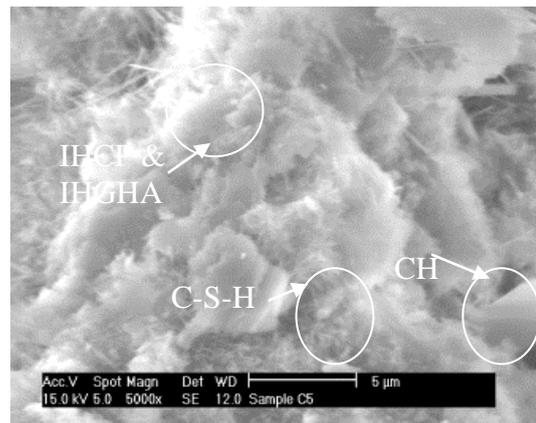
Fig. 4:SEM of 10% GHA-Concrete at 28 days
