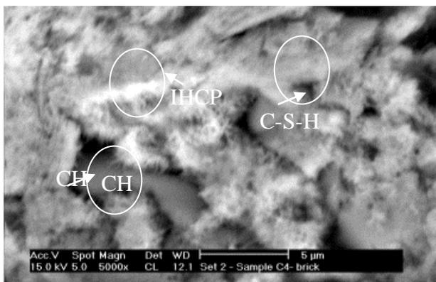
Fig. 5:SEM of OPC Concrete at 90 days,
