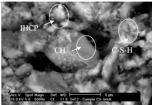
Fig. 3:SEM of OPC Concrete at 28 days,
