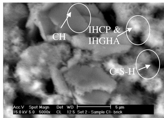
Fig. 6:SEM of 10% GHA-Concrete at 90 days
