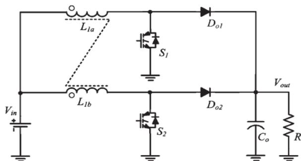
Figure 2.3: Interleaved boost converters with coupled inductor
