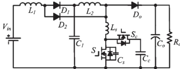
Figure 2.7: Integrated cascade boost converter with ZVS performance
