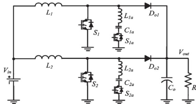
Figure 2.2: Active ZCT interleaved boost converter
