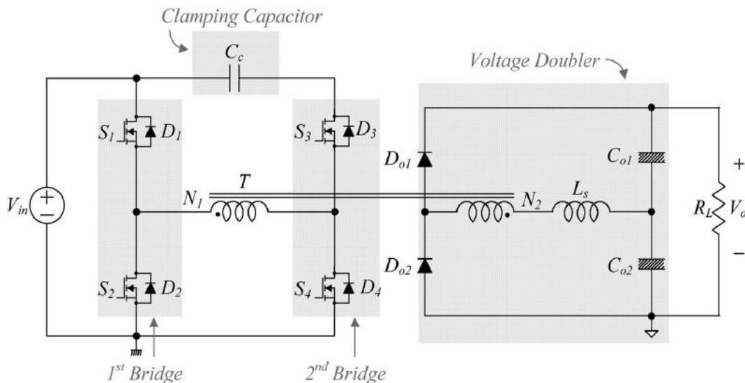
Figure 3.1: Circuit Diagram
