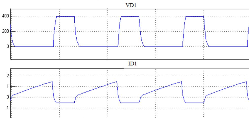
Figure 6.4: ZCS of Diode D1
