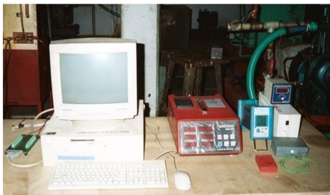
Figure.3. Photographic view of pressure and emissions measuring setup
