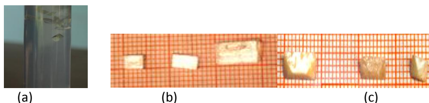
Fig.1:Photographs showing the (a)growing ST3 and ST4 crystals, (b)grown ST3crystals and (c)grown ST4 crystals
