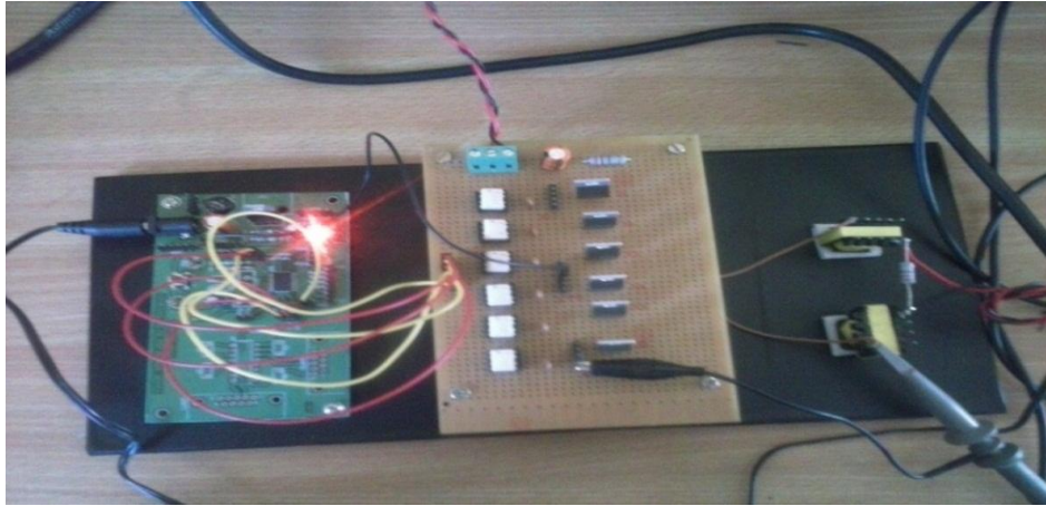
Fig: 10 Hardware implementation of H6 inverter
