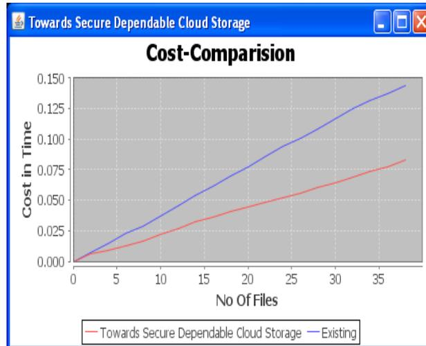
The following graph shown in Fig.1 is cost comparison graph in which, number of files ranging from 0 to 35 are taken along x-axis and cost time taken for upload file ranging from 0 to 0.15 minutes are taken along y-axis. It can be inferred from the graph that as like Encryption; Decryption time taken by Reed Solomon Erasure Code is lesser than existing System which indicates proposed system works faster than the existing system.
