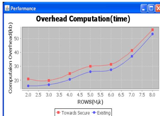
The following graph shown in Fig.2 is overhead computation graph in which, number of files ranging from 0 to 8 are taken along x-axis and overhead taken for distribute the file ranging from 10 to 50 kb are taken along y-axis. It can be inferred from the graph that as like Encryption; Decryption time taken by Reed Solomon Erasure Code is higher than existing System which indicates proposed system works faster than the existing system.
