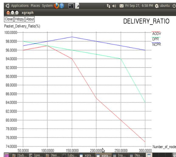
The Packet delivery ratio is shown in this graph. In the X-axis number of nodes is taken. Y-axis packet delivery ratio is taken. This graph clearly shows that the number of nodes is increases the packet delivery ratio is decreases in existing methods. But in the proposed coverage based probabilistic rebroadcast protocol, the packet delivery ratio is increases.
