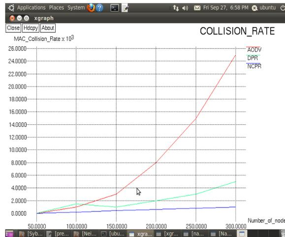
The Collision rate is shown in this graph. In the X-axis number of nodes are taken. Y-axis Collision rate is taken. This graph clearly shows that the number of nodes are increases the collision rate is increases in existing methods. But in the proposed coverage based probabilistic rebroadcast protocol, the collision rate is decreases.
