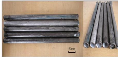
Figure 7 Composite tube of Al/Ti
