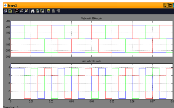
Fig.1.3. Three phase Load Current and Load Voltage waveform for inverter 180 0 mode of conduction without filter
