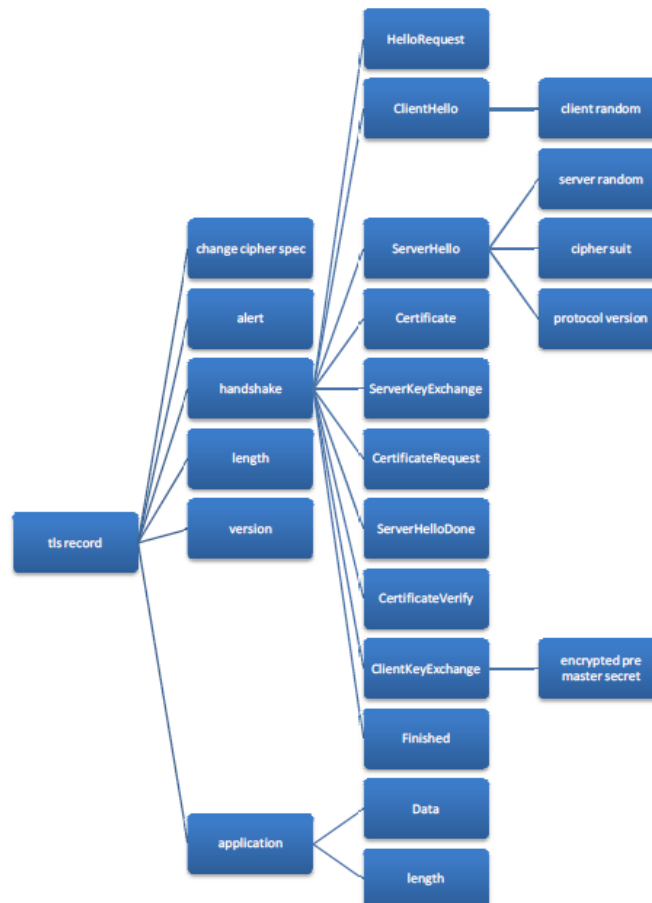
Fig 9. TLS Parser Design
