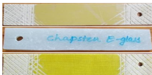
Fig. 5.5 Tensile Test Specimens of Glass Fiber Epoxy, Chapsten E-Glass Epoxy and Glass Fiber Polyester Epoxy
