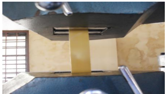
Fig. 5.4 Tensile Test in Process
