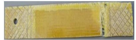
Fig. 5.6 Glass Fiber Epoxy Specimen after Tensile Test Fig. 5.7 Chapsten E-Glass Epoxy Specimen after Tensile Test Fig. 5.8 Glass Fiber Polyester Epoxy Specimen after Tensile Test
