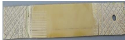
Fig. 5.6 Glass Fiber Epoxy Specimen after Tensile Test Fig. 5.7 Chapsten E-Glass Epoxy Specimen after Tensile Test Fig. 5.8 Glass Fiber Polyester Epoxy Specimen after Tensile Test
