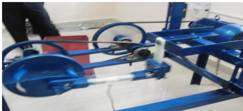
Fig. 2.1 Schematic Diagram of Fatigue Test Rig
