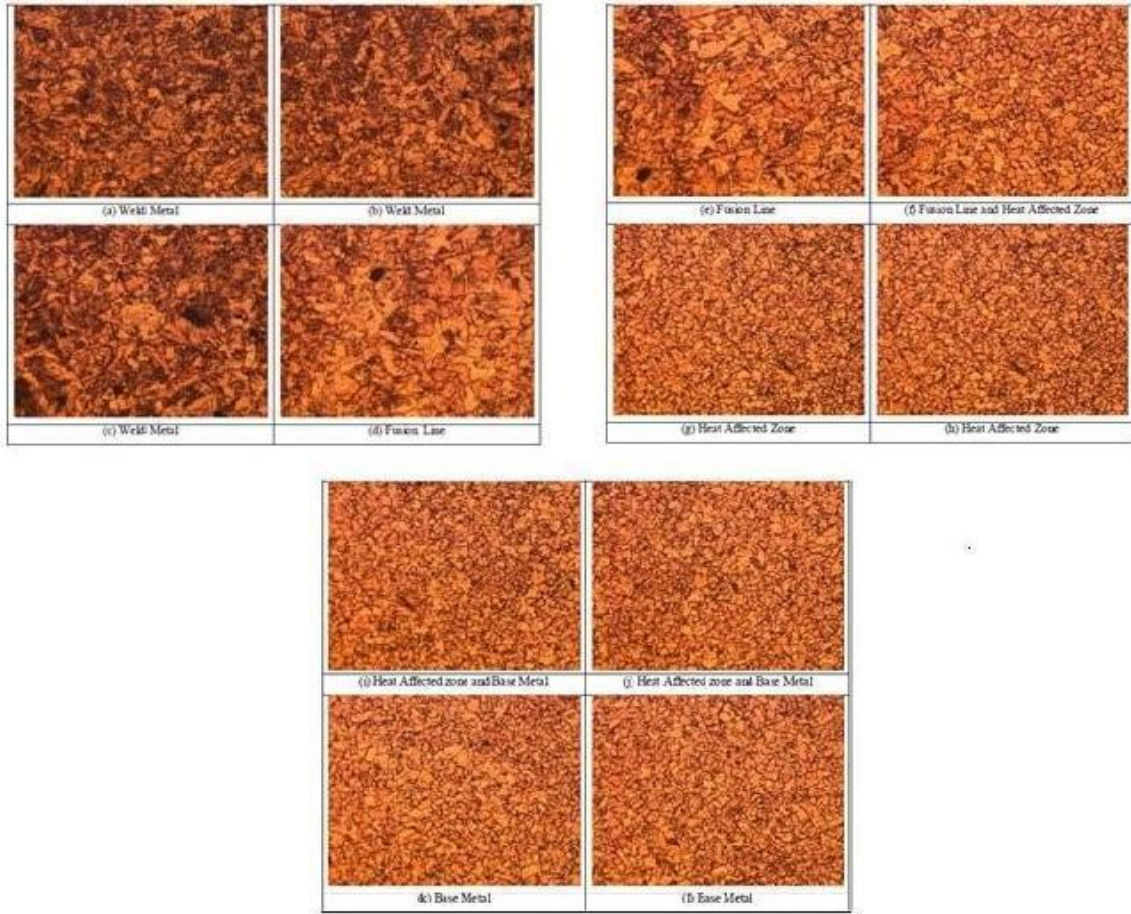
Figure : 5 Microstructure with heat input = 1547.98J/mm
