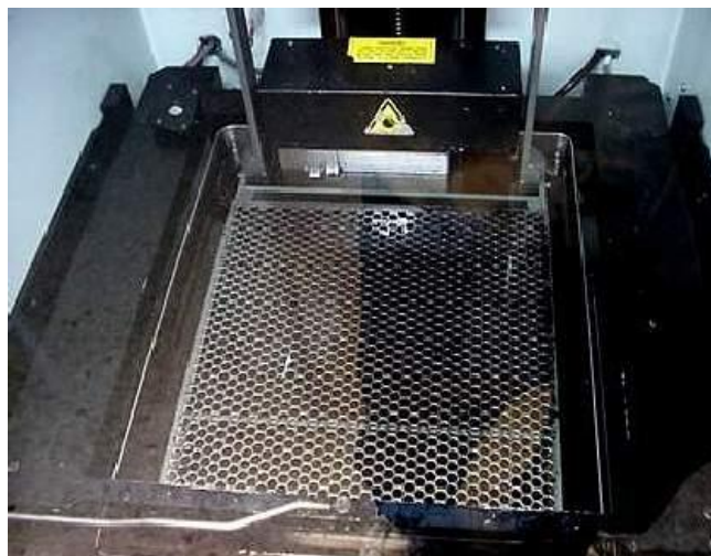
The platform in the tank of photopolymer at the beginning
