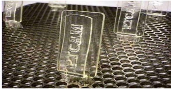
The platform at the end of a print run, shown here with several identical objects
