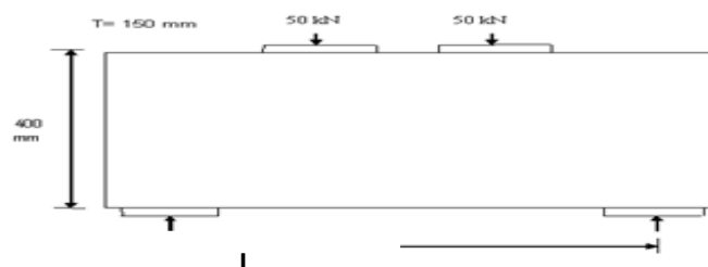
Fig. 1 Deep beam with two point loads
