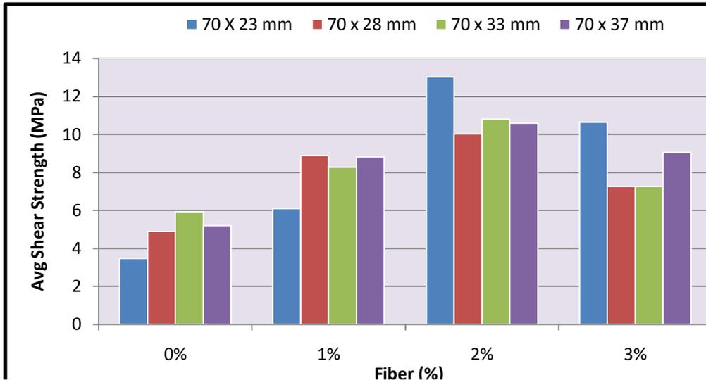
FIG.3.0: SHEAR STRENGTH OF RPC WITH STEEL FIBRE VARIATION
