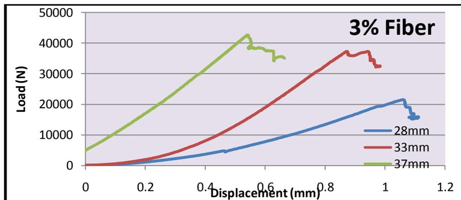
FIG.8.0: EFFECT OF 3.0% STEEL FIBER IN DIFFERENT SHEAR DEPTH
