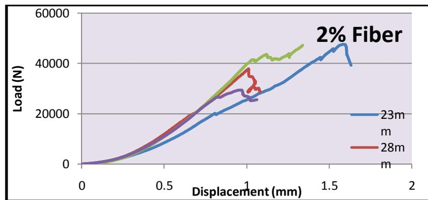
FIG.7.0: EFFECT OF 2.0% STEEL FIBER IN DIFFERENT SHEAR DEPTH
