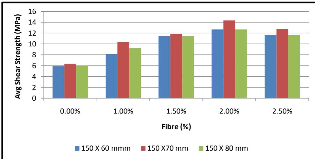
FIG: 4.0 SHEAR STRENGTH OF RPC WITH STEEL FIBRE VARIATIONS.
