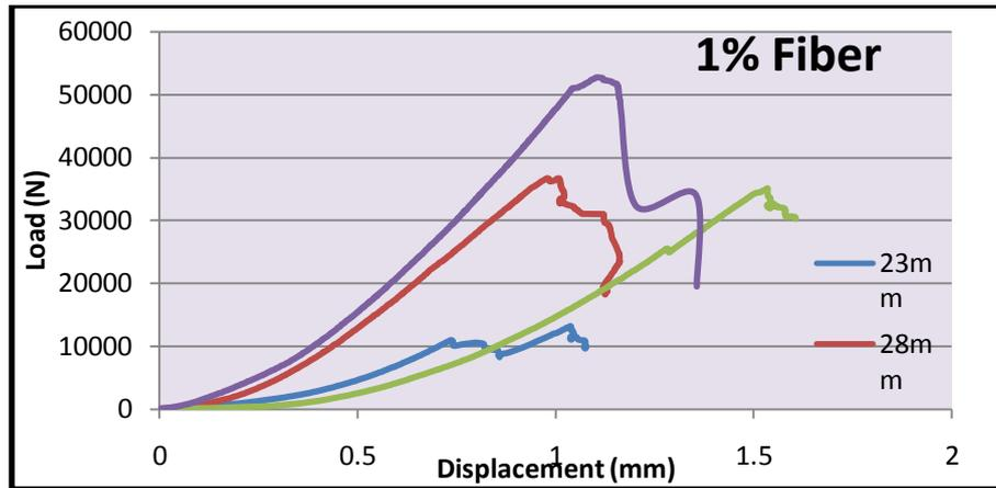
FIG.6.0: EFFECT OF 1.0% STEEL FIBER IN DIFFERENT SHEAR DEPTH
