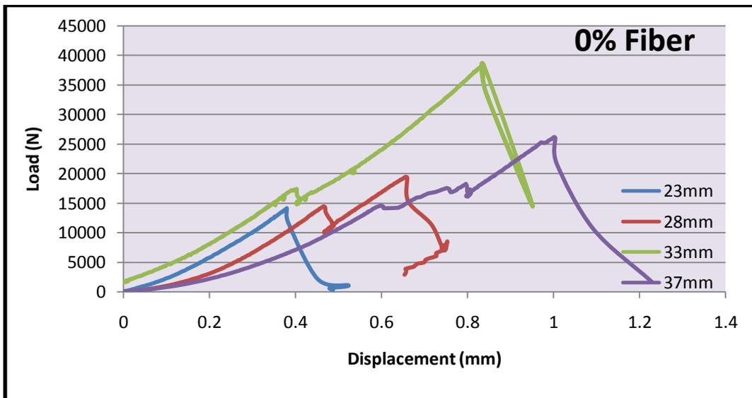
FIG.5.0: EFFECT OF 0.0% STEEL FIBER IN DIFFERENT SHEAR DEPTH
