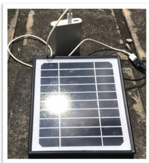
Figure 3. Charging the portable power bank using the solar panel
