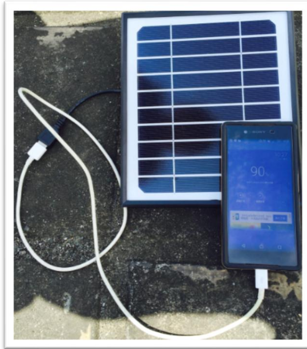
Figure 4. Charging a mobile phone using the solar panel
