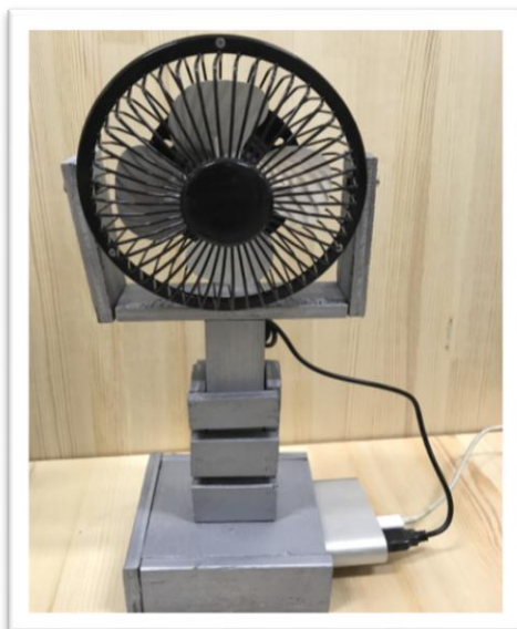
Figure 2. Platform for placing the fan and portable power bank
