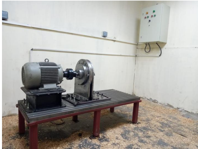
Figure 7: Power transmission elements test rig
