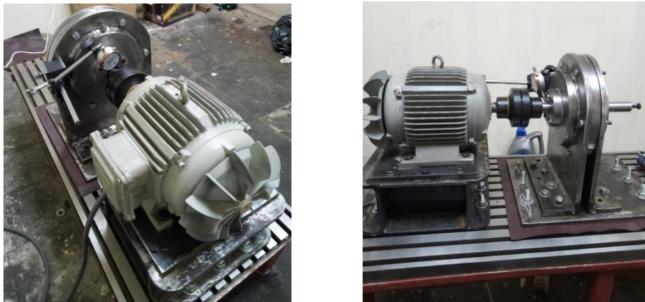
Figure 6: Alignment of connecting shafts of planetary gearbox
