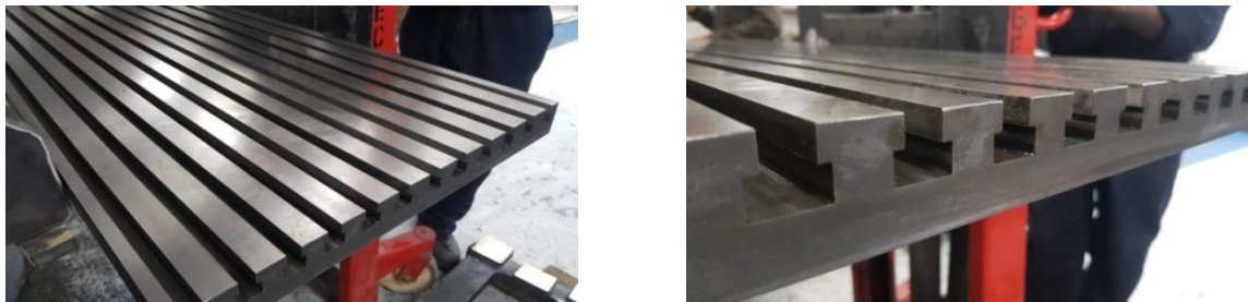
Figure 4: Manufactured T-Slot base plate
