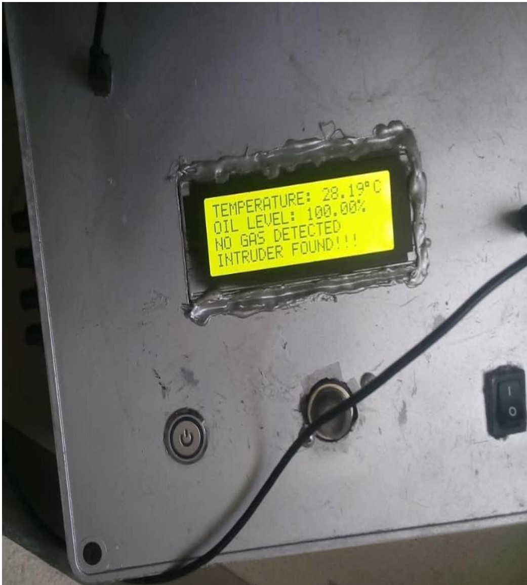
Plate 3: When Gas is not Detected, Intruder is Detected, Temperature is 28.19°C and oil level is 100.00%
