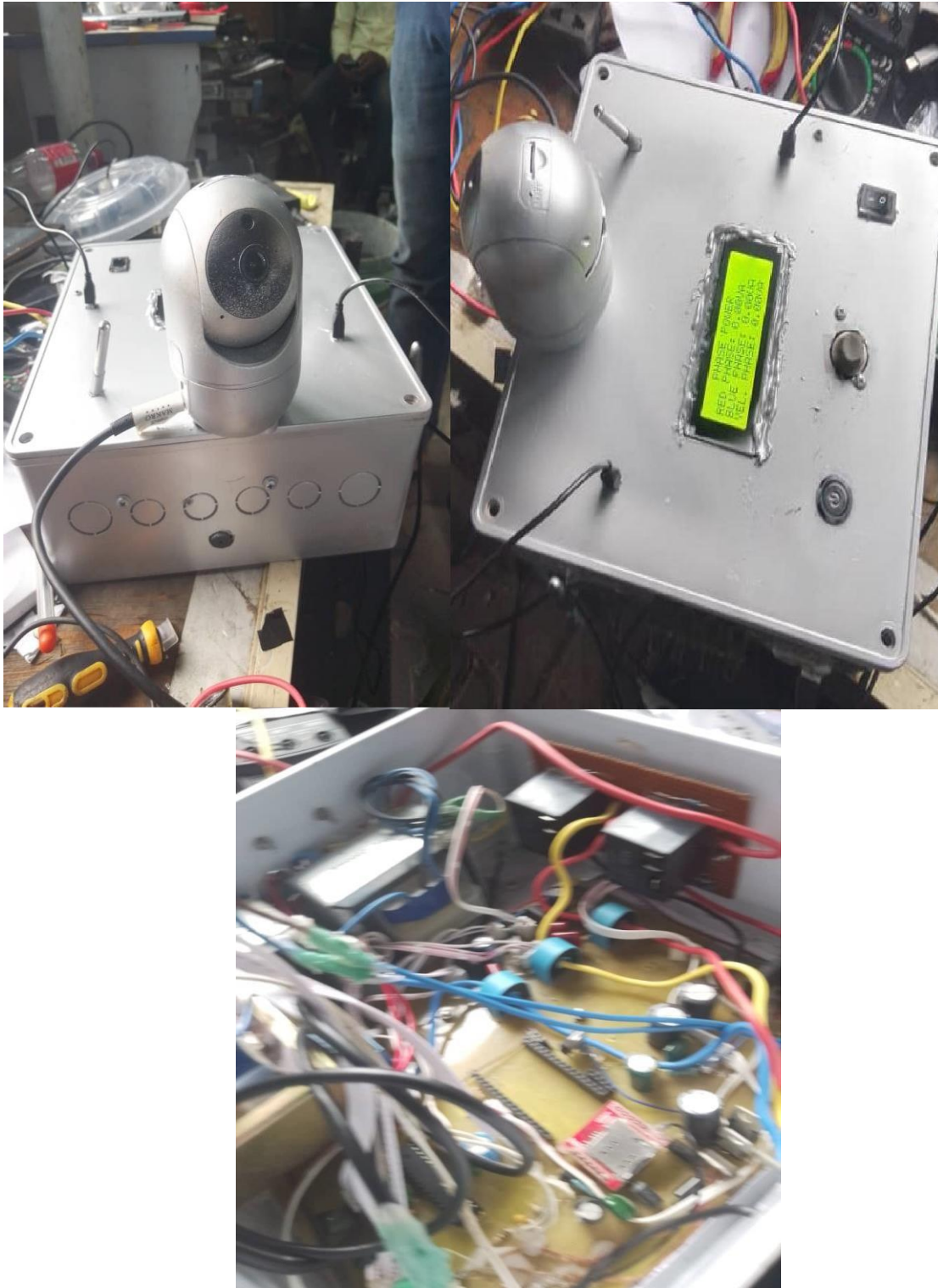
Fig. 4: Complete hardware implementation of the GSM and IoT-based transformer monitoring system
