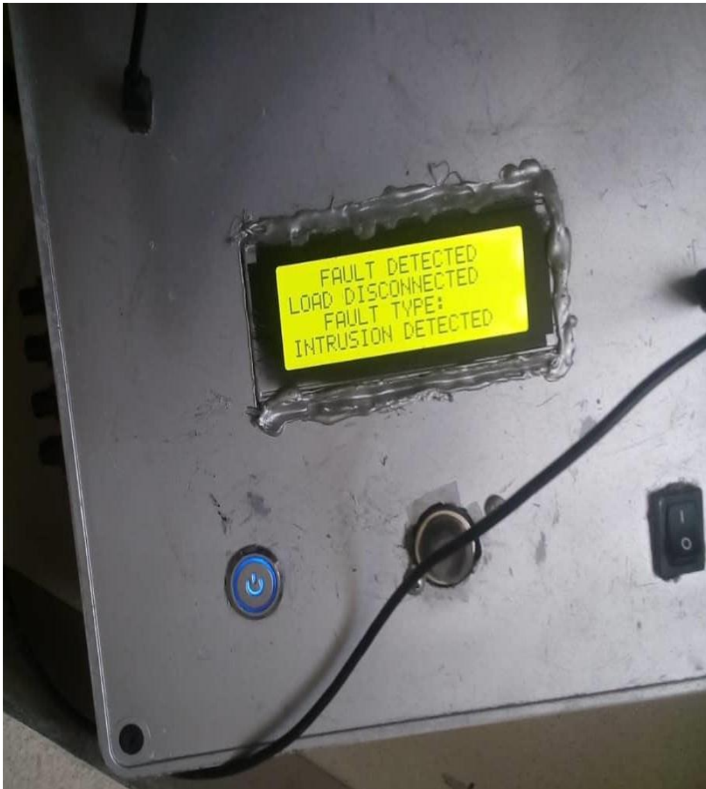
Plate 4: When Fault is Detected, Load is Disconnected and Fault Types is Intrusion
