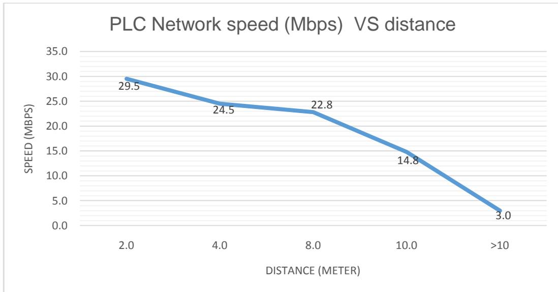
Figure(2):PLC Network speed (Mbps) VS distance
