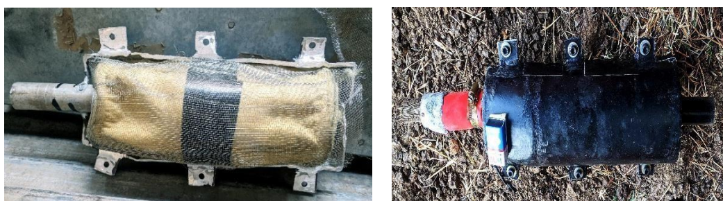
Fig.13: Inner packaging, mounting and assembly of Catalytic Converter
