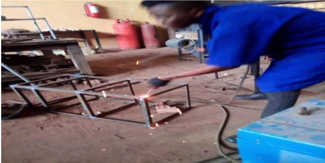
Plate 3: Body Frame Welding process.
