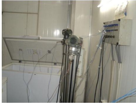
Fig.4 Freezer connected with Pressure gauges and Thermocouples
