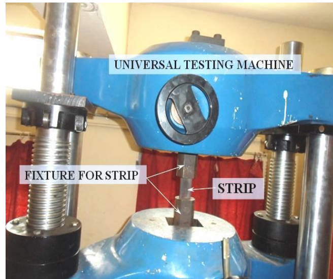
Fig.3 Testing of Chain strip
