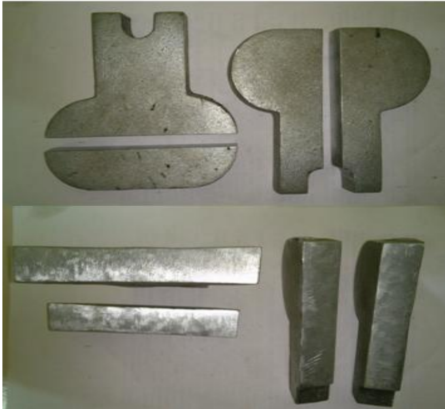
Fig. 17. section cut of casting with feeder of diameter 50mm and sleeve thickness 10mm shows no defects
