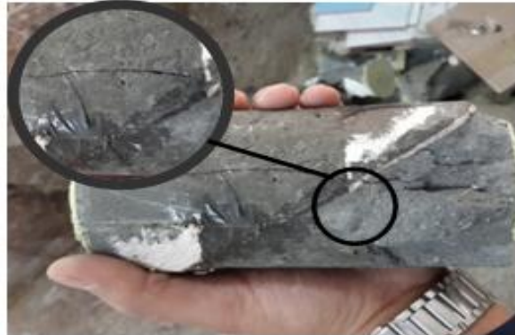
Fig.11. The bond strength of polymer-mortar.
