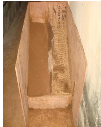
Figure. 6. Landslide model constructed in the laboratory
