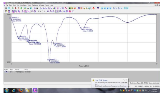
Fig15:Return loss of design with 2 U-slots and slot rotated to 90°
