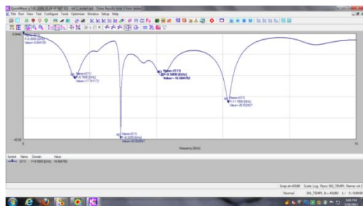
Fig19:Return loss of design with 2 U-slots and slot rotated to 180^\circ
