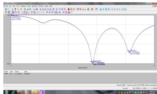
Fig9: Return loss of design with 1 U-slot
