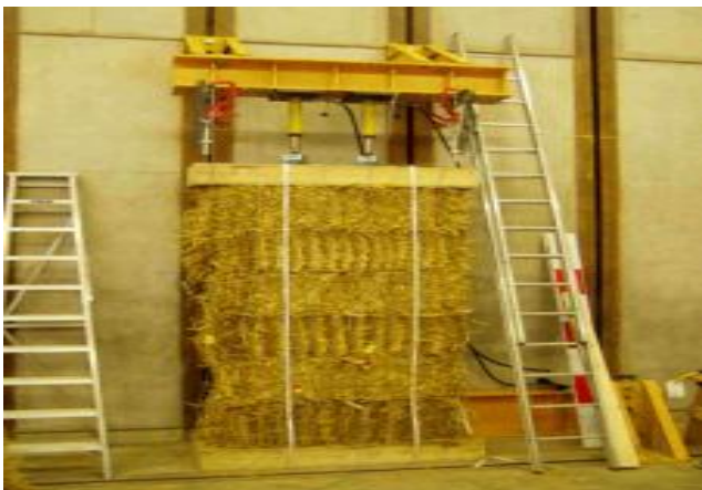
Fig 4. Static load test
