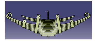
Fig 1.Solid Model of multi-plate leaf spring
