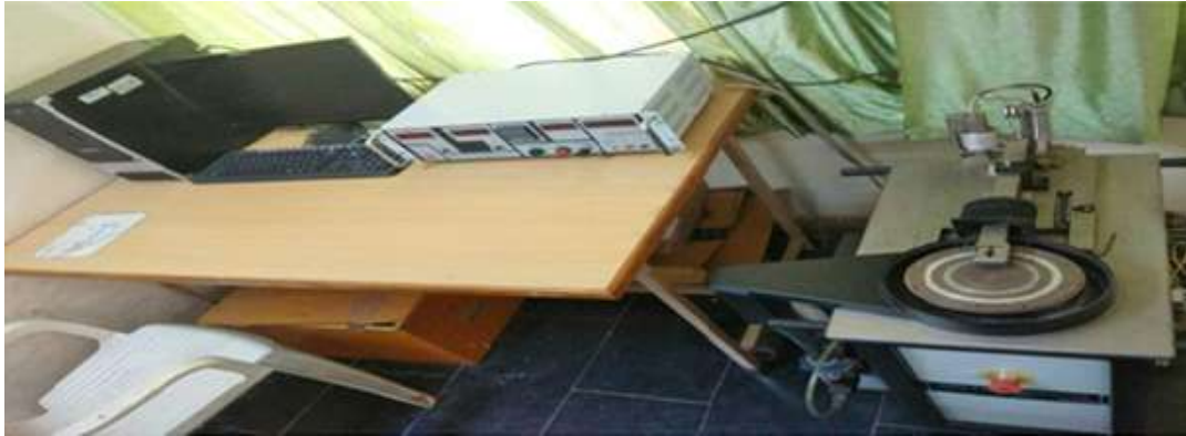
Fig 2: (a) Specimens before testing (b) Fig: Pin-on-disc wear testing Machine
