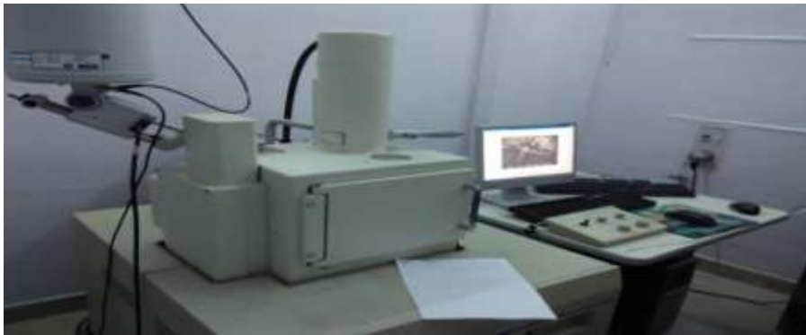
Figure 3: The Scanning Electron Microscope used for Microstructure study B 4 C Particles
