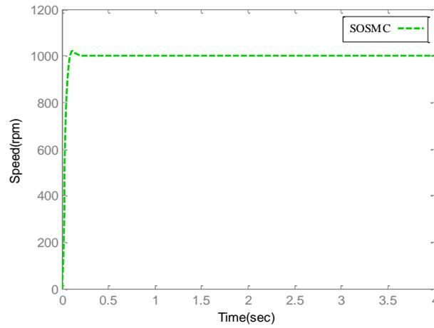
Fig.5. Response to speed change (0-1000 rpm)
