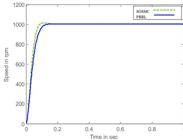
Fig.15 Combined result of SOSMC & PRRL for speed
