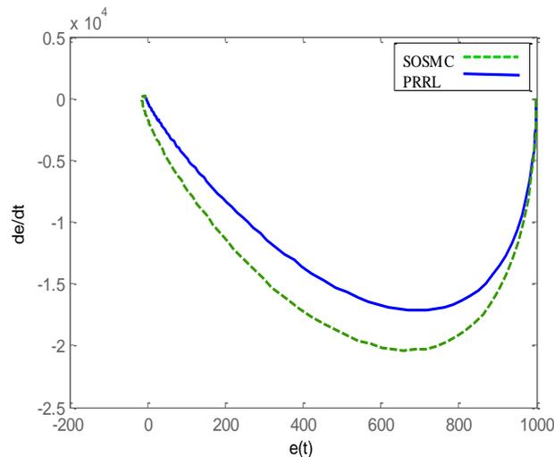
Fig.17 Combined result OF SOSMC & PRRL for phase trajectory.
