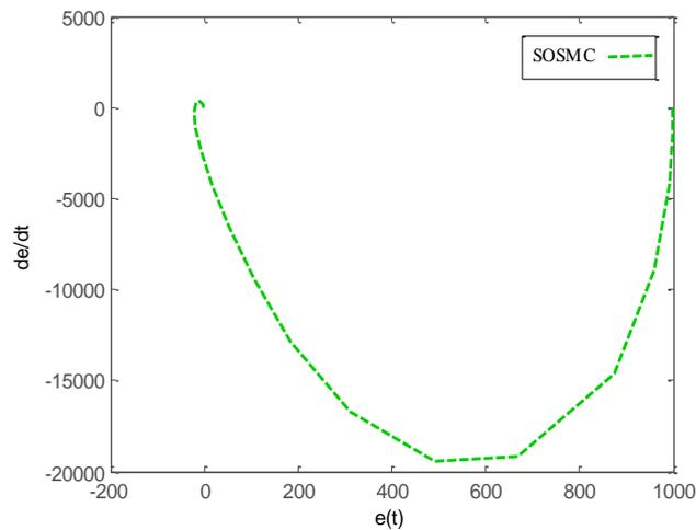
Fig.7. The phase plane trajectory of the 2-SMC system
