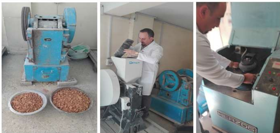
Plate 1. Step's of crushing and grinding the WCBs
