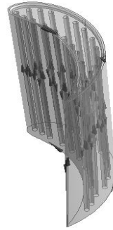
Figure 3.8 Cooling Design from root to tip
